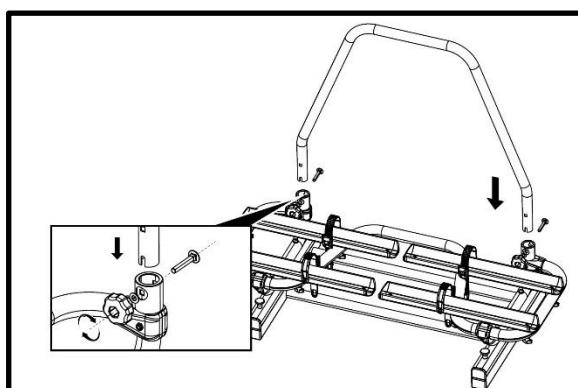
Secure this U-tube with the supplied carriage bolts (M8x60), washers and plastic rotary knobs. Make sure the plastic rotary knobs are on the frontside (see drawing).
