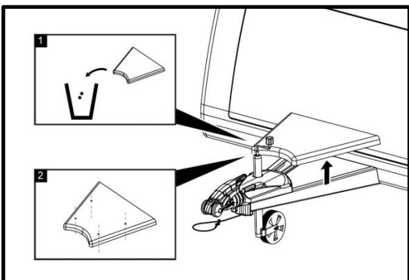
Remove the A-frame cover from the A-frame (1) or drill holes in the A-frame cover for the U-bolts (2).
