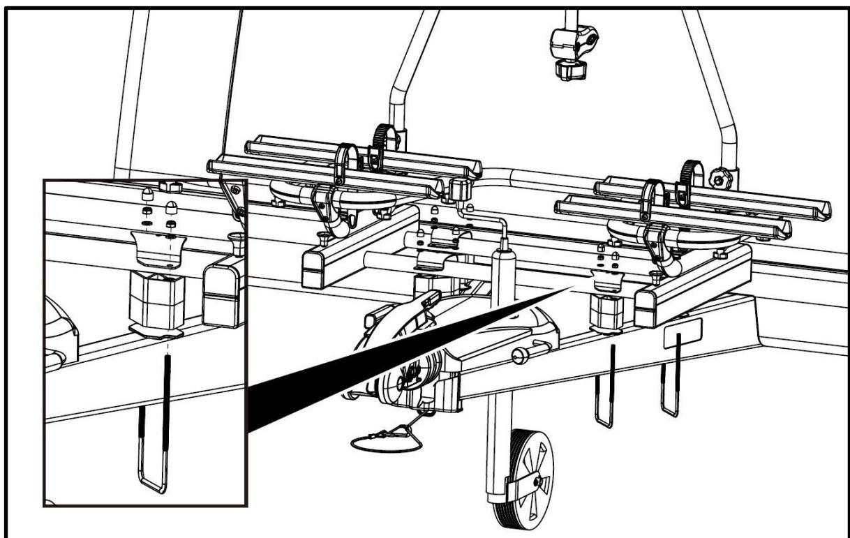
To make sure that the carrier remains in its position, it must be secured with the four screws. To do so, 4 small holes (3 mm) must be drilled in the base part, after which the clamp and the base frame can be screwed together.
